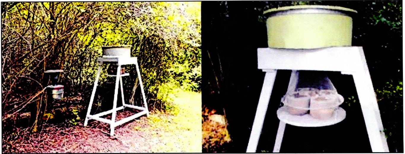
Fig. 1. Stationary insect collection traps with attached collection chamber.
