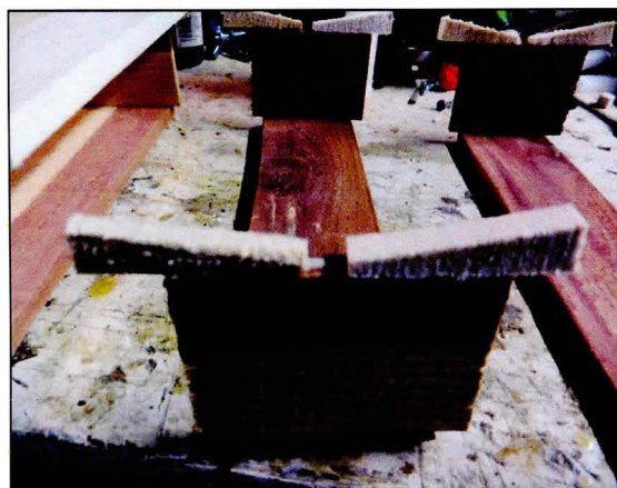
Fig. 2. Trailing Edge slices glued upright end boards.
