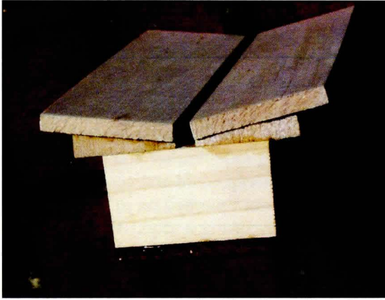
Fig. 4. End view of smaller Trailing Edge glued to smaller spreading boards.
