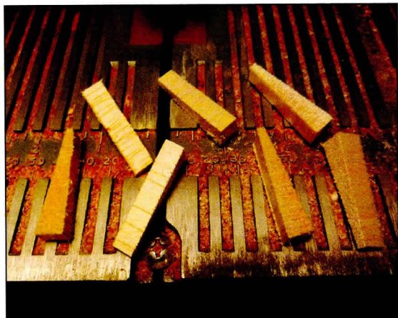
Fig. 1. Slices of Trailing Edge used to give the proper angle to spreading boards.
