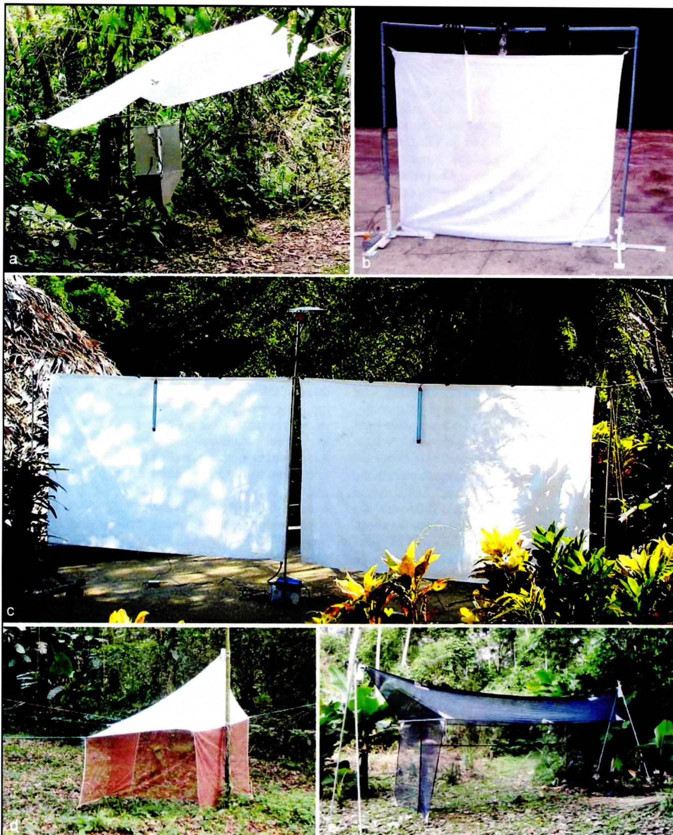
Fig. 1. Traps and light sheet arrangements: a) UV light trap under rain canopy, with square funnel and designed to be disassembled for easy transport; plastic bag and collecting bucket would go beneath and the bag is attached to the rim of the funnel with plastic report binders (in Peru); b) self-standing light sheet arrangement, with MV and UV lights (in Korea); c) large light sheet arrangement with ropes tied to nearby trees or other supports, with 250-watt metal halide central light and 15-watt UV lights (in Guatemala); d) Townes-type 2m-flight trap (in Guatemala); e) large 6m-flight trap with cups at both ends, supported by 2.5m (8 foot) high poles at each end and tied to nearby trees (in Peru).
