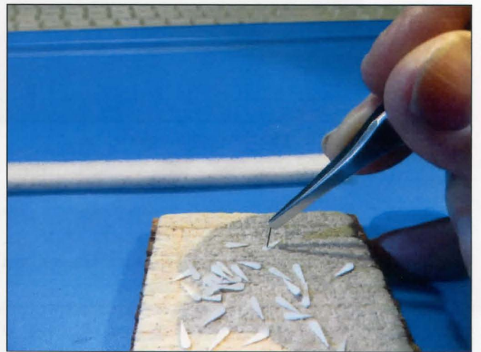
Fig. 9. Inserting sheared pins into points on soft balsa block.
