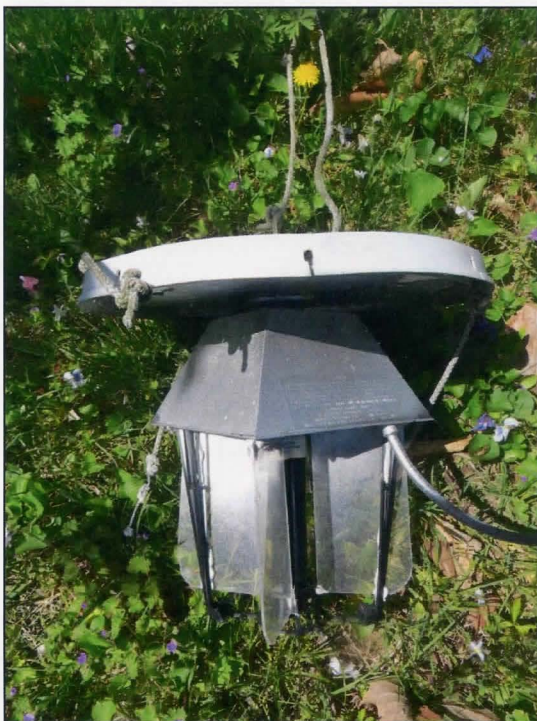
Fig. 1. Late iteration of UV Bug Zapper converted to moth trap with 4 clear plastic vanes and ropes to hang plastic bucket with funnel underneath.
