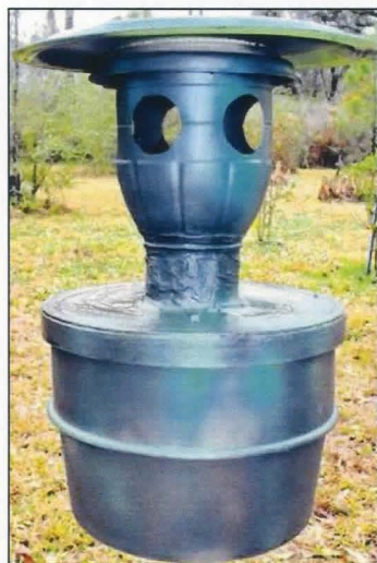
Fig. 3. Trap with 10" diameter collection chamber.
