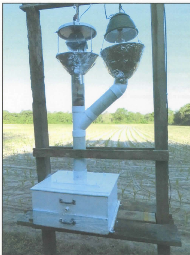
Fig. 1. Double UV collecting station with drawers for specimens to collect in, later modified to have UV and HG.
