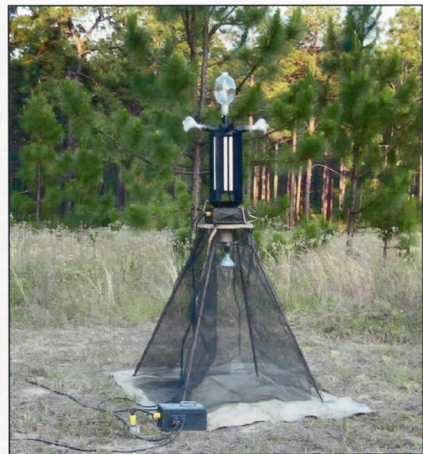
Fig. 8. Example of one of the light traps used on field trips across Louisiana
