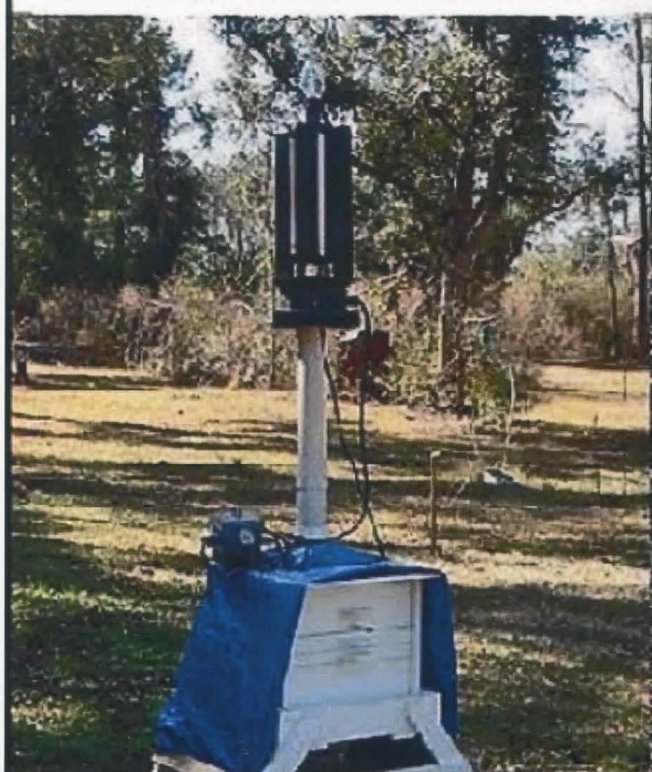
AESS light trap #3. (1) 175-watt mercury vapor lamp, and (4) 15-watt fluorescent blacklights.
