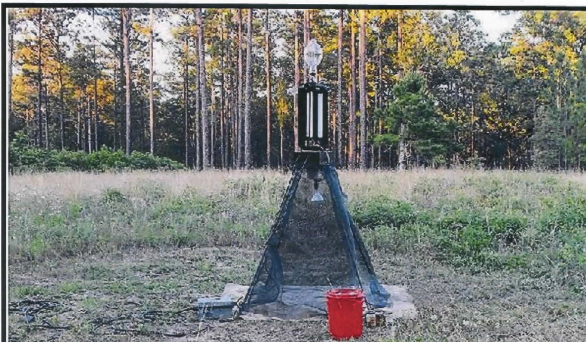
AESS, live-capture Light trap #8 . (1) 1000-watt mercury vapor lamp, and (2) 275-watt RS sunlamps, and (8) 15-watt fluorescent blacklights, and (1) 160-watt mercury vapor lamp
