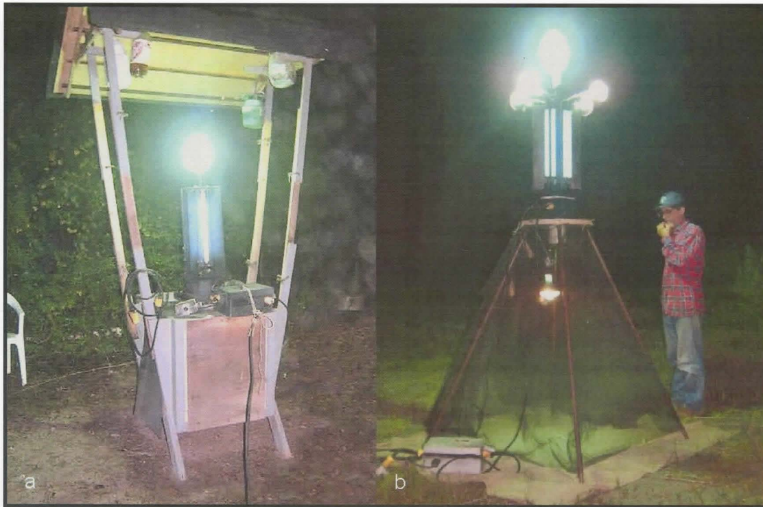
Fig. 13. a. Light trap (1) 400 watt mercury vapor lamp and (4) 15-watt fluorescent blacklights and collection chamber, one sesiid lure trap at the AESS, b. Light trap (1) 1000-watt mercury vapor lamp, and (5) 275-watt RS sunlamps, and (8) 15-watt fluorescent blacklights, used for fieldwork and occasionally at the AESS.
