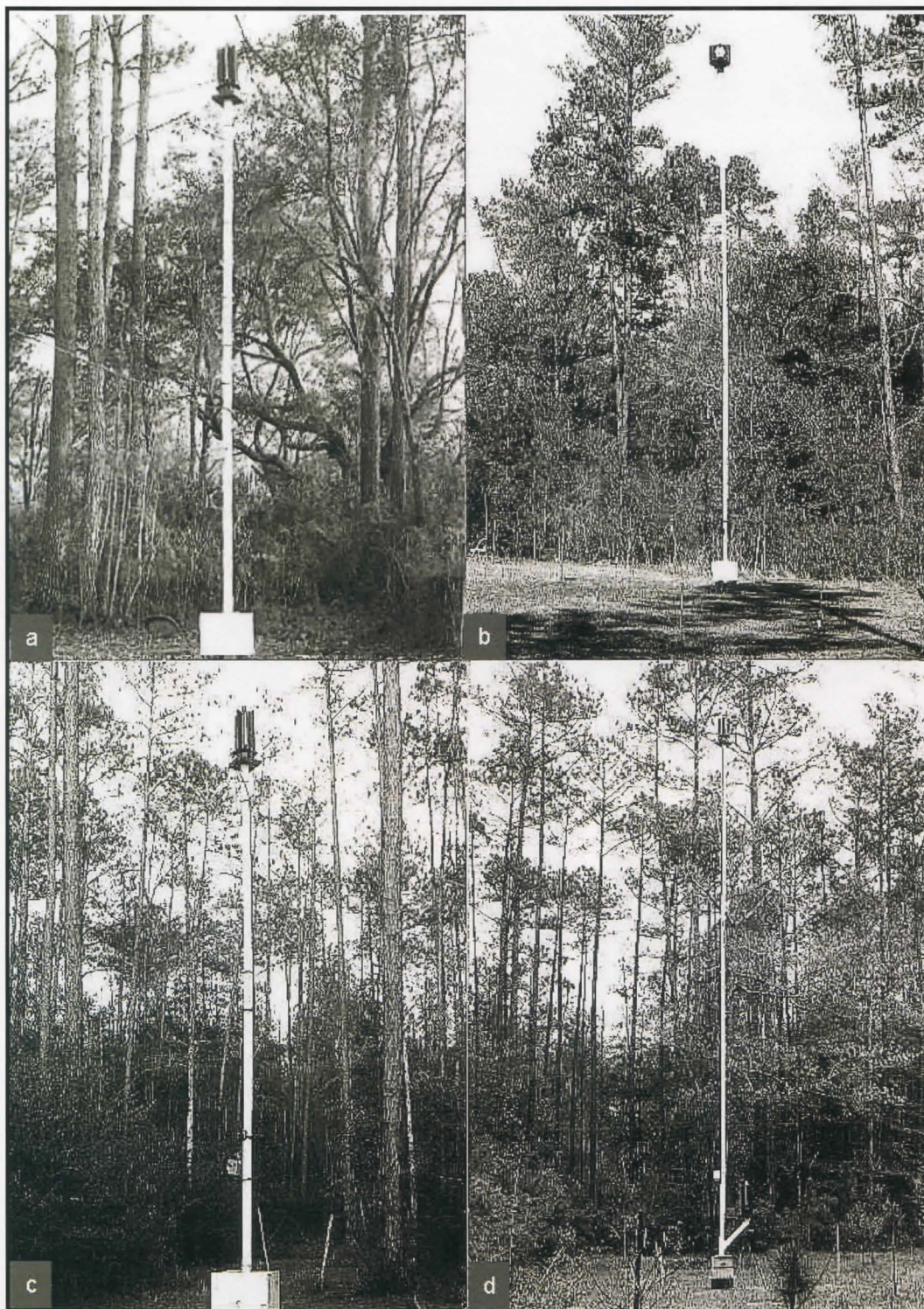
Fig. 5. Examples of light traps operated above secondary lower growth vegetation at the AESS in the 1980s. a. 175-watt mercury vapor lamp with (4) 15-watt blacklight fluorescent tubes, trap 8-meters above ground, b. 1000-watt mercury vapor lamp, trap 16-meters above ground, c. 400-watt mercury vapor lamp, trap 8-meters above ground, d. upper trap 16-meters above ground 175-watt mercury vapor lamp with (4) 15-watt blacklight fluorescent tubes, lower trap 2-meters above ground 175-watt mercury vapor lamp with (4) 15-watt blacklight fluorescent tubes, all traps fitted with NaCn dispatching wooden automatic-capture collection chambers.
