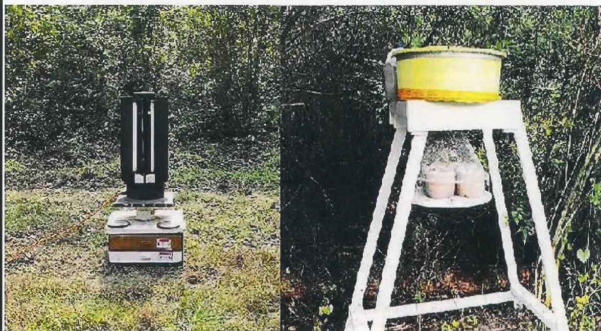
AESS Left: Light trap #9 . (4) 15-watt fluorescent blacklights, and (1) 160-watt mercury vapor lamp with collection chamber, right: Fermenting fruit bait trap #4 with automatic capture collection chamber.
