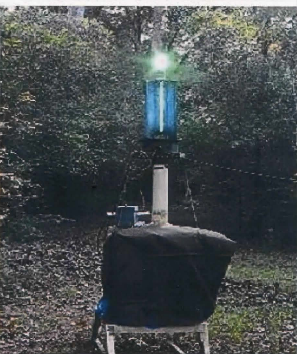
AESS light trap #4. (1) 175-watt mercury vapor lamp, and (4) 15-watt fluorescent blacklights.
