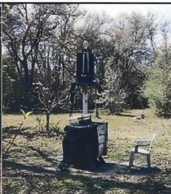
AESS light trap #2. (1) 400-watt mercury vapor lamp, and (4) 15-watt fluorescent blacklights.
