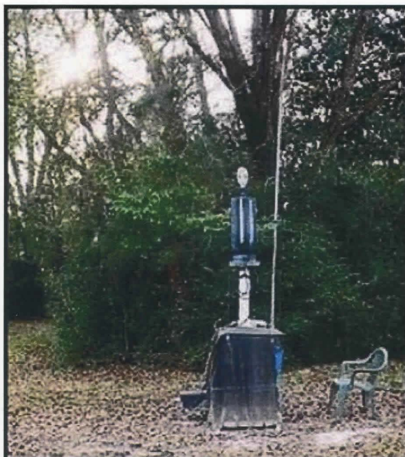
AESS light trap #1. (1) 400-watt mercury vapor lamp, and (4) 15-watt fluorescent blacklights.
