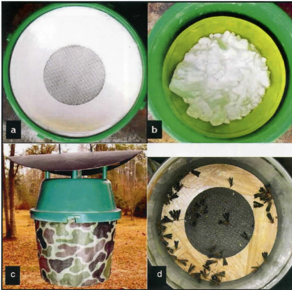
Fig 4. Revised 'Unitrap' bucket trap with a. screened bottom basket insert, b. container of sodium cyanide briquettes/granules below basket insert, c. ready for field placement with added accoutrements, including larger rain/sun/heat shield, d. dispatched captured clearwing moths in basket insert.
