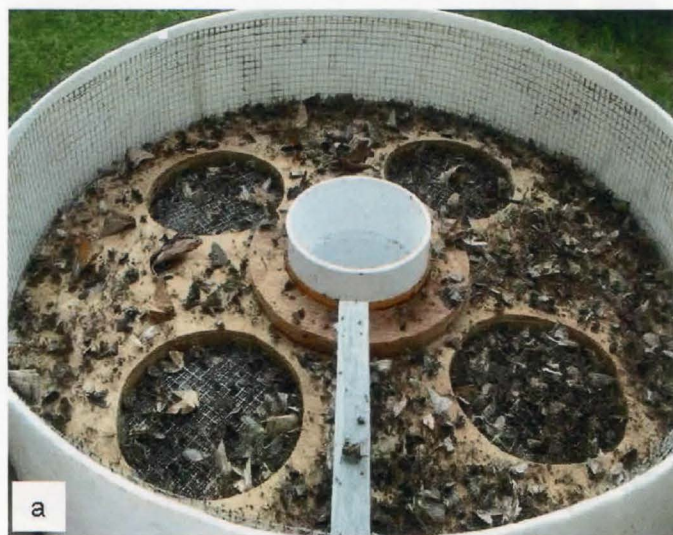
Fig. 7. The same concept 'gravity based automatic light trap wooden collecting chamber' can be applied to many other types of insect traps as we illustrate here a. lid removed from automatic collection chamber where insects are guided upwards into killing chamber via inverted funnel on fermenting fruit-based bait traps and NaCn or KCn are the dispatching agents, b. example of gravity based clearwing moth traps where lures are placed inside of upper entrance area and moths are gravity fed into the collecting chamber below using NaCn or KCn as the dispatching agents, c. captured moths inside of collecting chamber.
