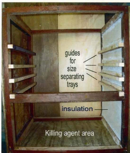
Fig. 3. Front view. Beginning of fabrication for 4-drawer automatic light trap wooden collecting chamber. This basic concept trap chamber operated successively and continuously 365-366 days for each of the past 55 years.
