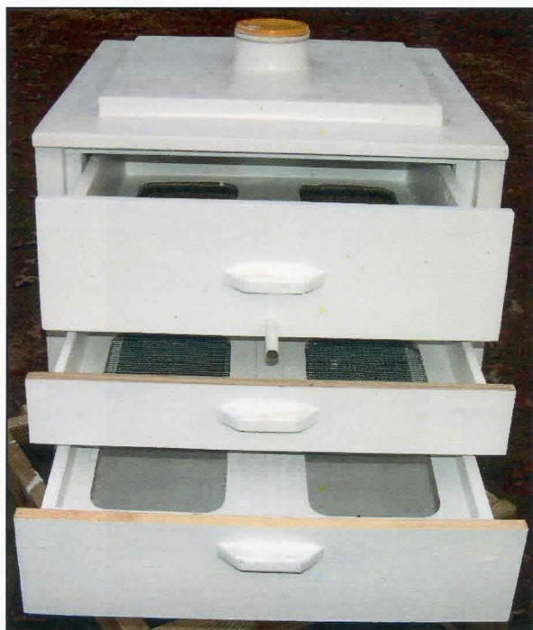
Fig. 2. Front view. Newly fabricated 3-drawer automatic light trap wooden collecting chamber. This basic concept trap chamber operated successively for each of the past 55 years.
