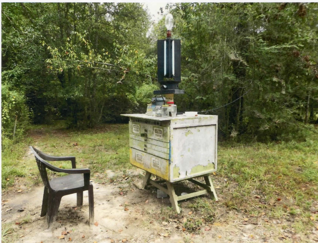
Fig. 6. 4-drawer automatic light trap wooden collecting chamber operating in the field across Louisiana.
