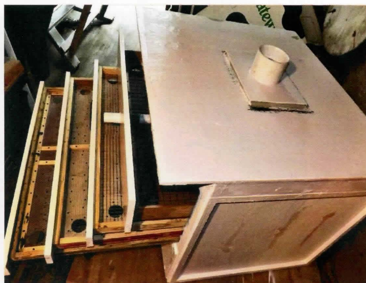
Fig. 4. Side view from above. Newly fabricated 4-drawer automatic light trap wooden chamber designed in 1969. This basic concept trap operated successively and continuously 365-366 days for each of the past 55 years.
