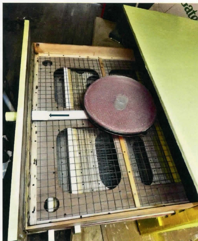
Fig. 5. Upper view. 4-drawer Newly fabricated automatic light trap wooden collecting chamber illustrates first upper of 4-drawer collection chamber pulled out to reveal rain drain and drain tube exiting out to front of drawer. This basic concept wooden collecting chamber operated for the past (55 years) 1969 to 2024 across Louisiana.
